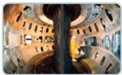
Interior of DIII-D Tokamak plasma reaction chamber
