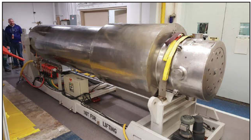
The shipping cask with "sister" fuel rods after it arrived at Oak Ridge National Laboratory in early 2016. Researchers will compare the physical state of the sister rods with the rods inside the modified Areva TN-32B dry storage cask after a decade of storage. (Photo: DOE/ORNL)
