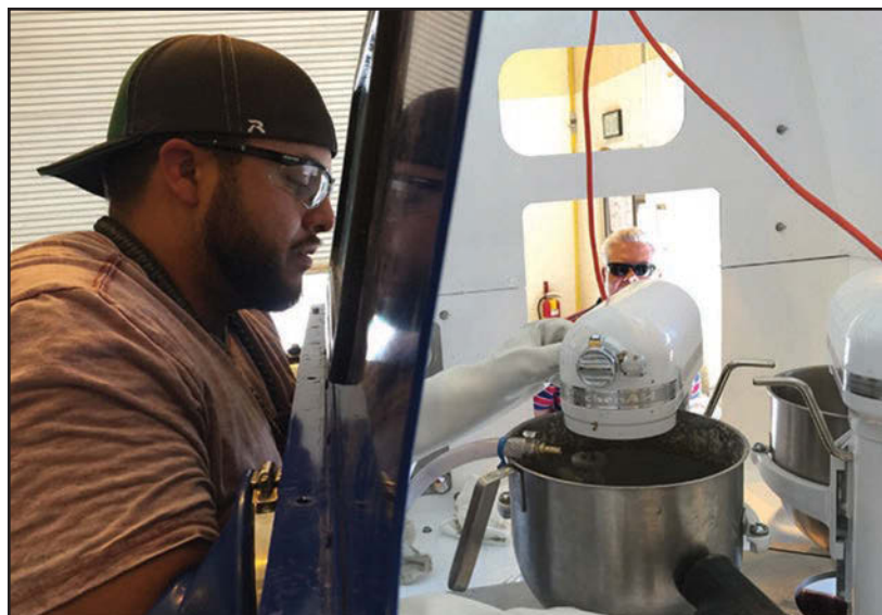
LANL technicians practiced and refined the method for treating remediated nitrate salts using a mock-up glovebox closely resembling the glovebox used during the actual treatment. (Photo: DOE)
