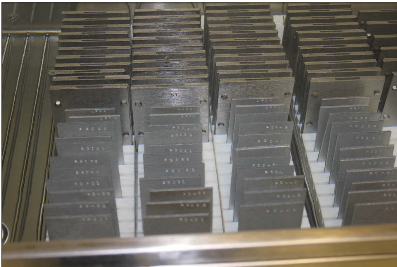
Fig. 2. Bare (front) and SS-encapsulated (back) Boral coupons in a test bath.
