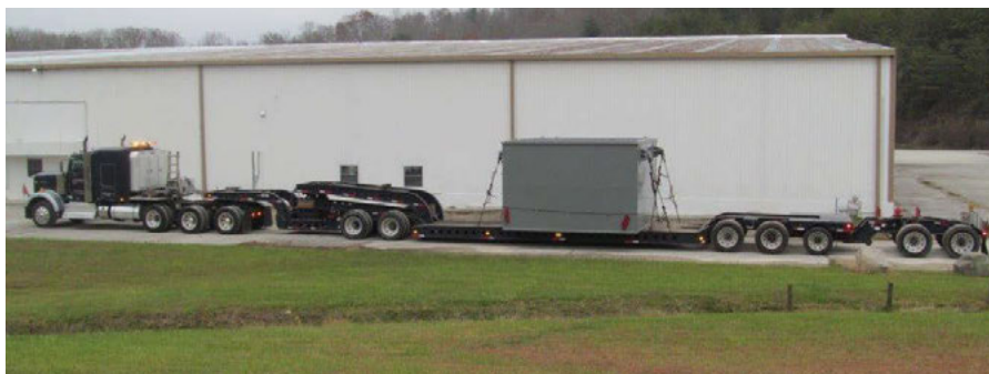
Shielded LCA Container 4" Plate 111,000 lbs Tare Weight
