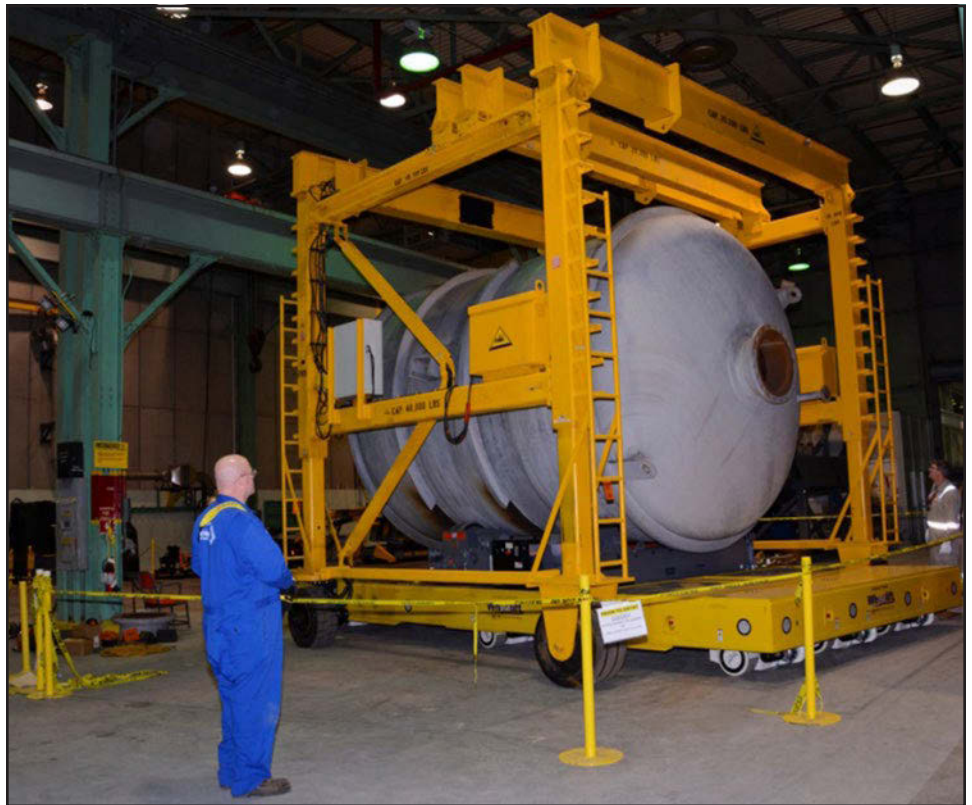
Remote-controlled straddle carriers will be used to handle converter components and eliminate the reliance on aging building cranes.
