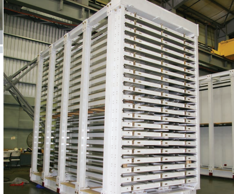
Rod Storage Rack – Shaw Areva MOX Services
