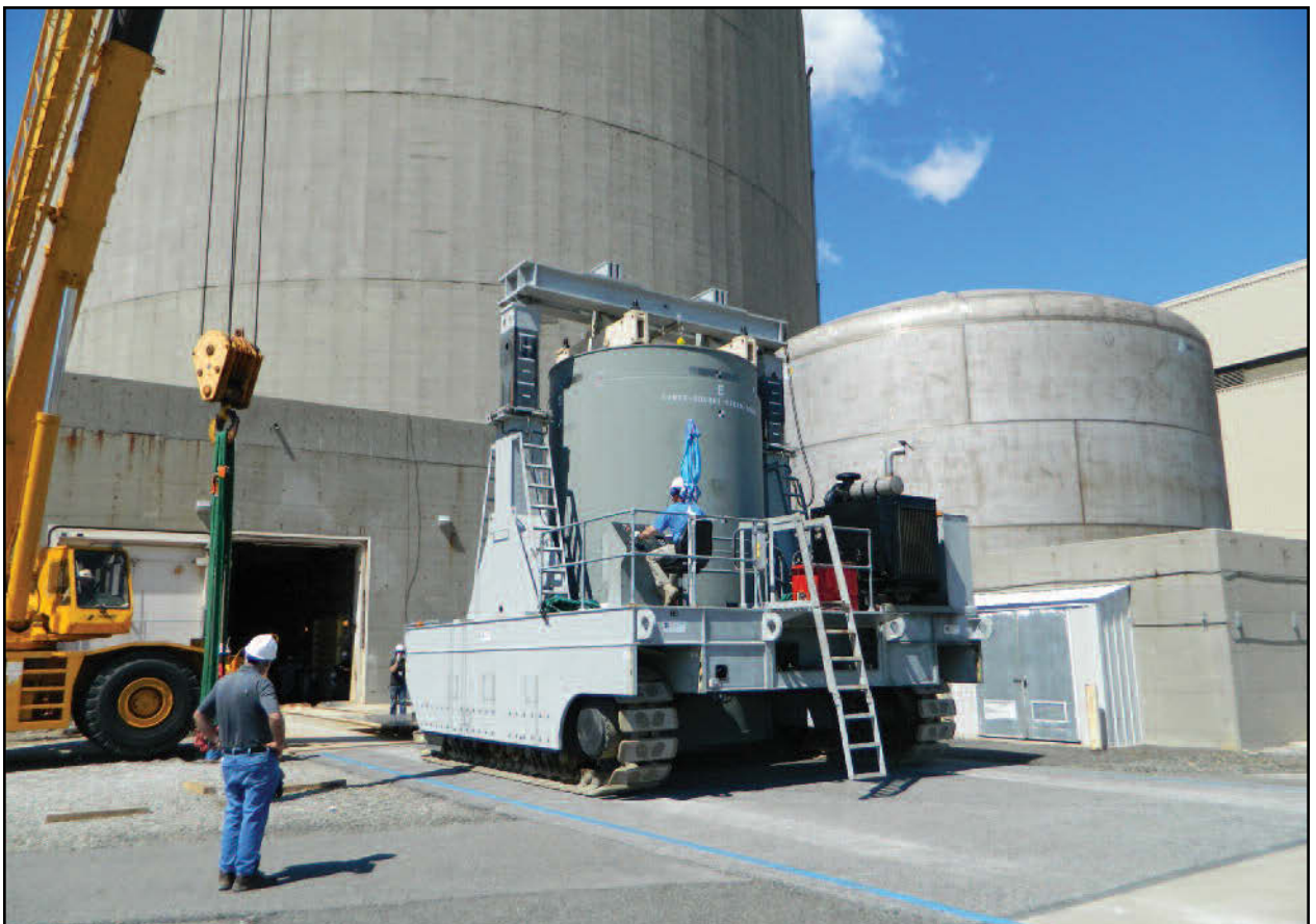
The cask is then placed onto a vertical cask transporter (VCT).
