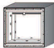
INTERNAL EXPANSION AIRFLOW RATED 3hr FIRE DAMPER
