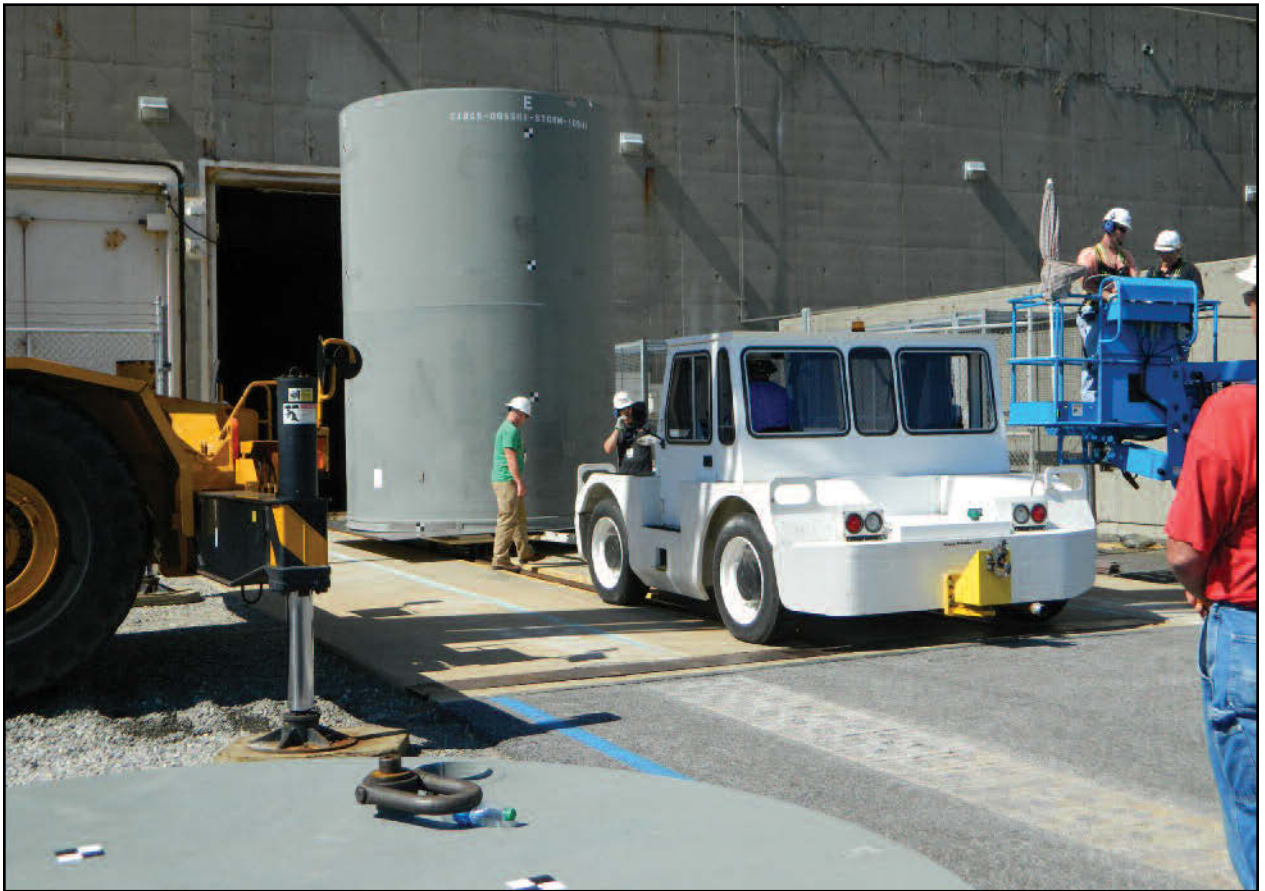
A loaded HI-STORM cask is moved out of the truck bay.
