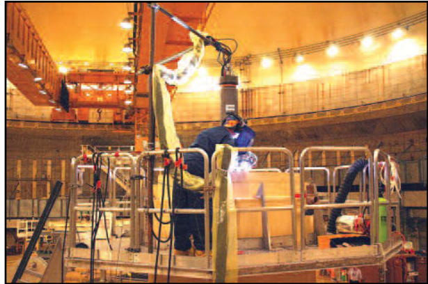
After being loaded, a multipurpose canister is welded shut.
