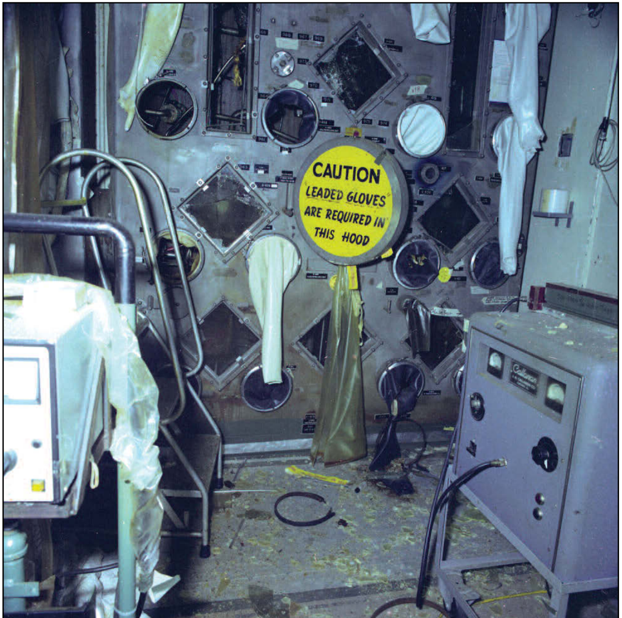
In this photo taken shortly after the 1976 incident, shards of plastic and glass on the floor of the McCluskey Room at Hanford's PFP can be seen near the glove box in which there was an explosion after nitric acid was added to an ion exchange column containing resin and americium. The force from the explosion blew the gloves from the glove box outward into the room. (Photos courtesy of CH2M Hill Plateau Remediation Company)
