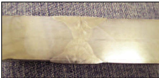
Fig. 4. The as-received flat-plate welds, November 2013. A section of the flat-plate weld (inset) was cut for microstructural analysis from the end of each weld.
