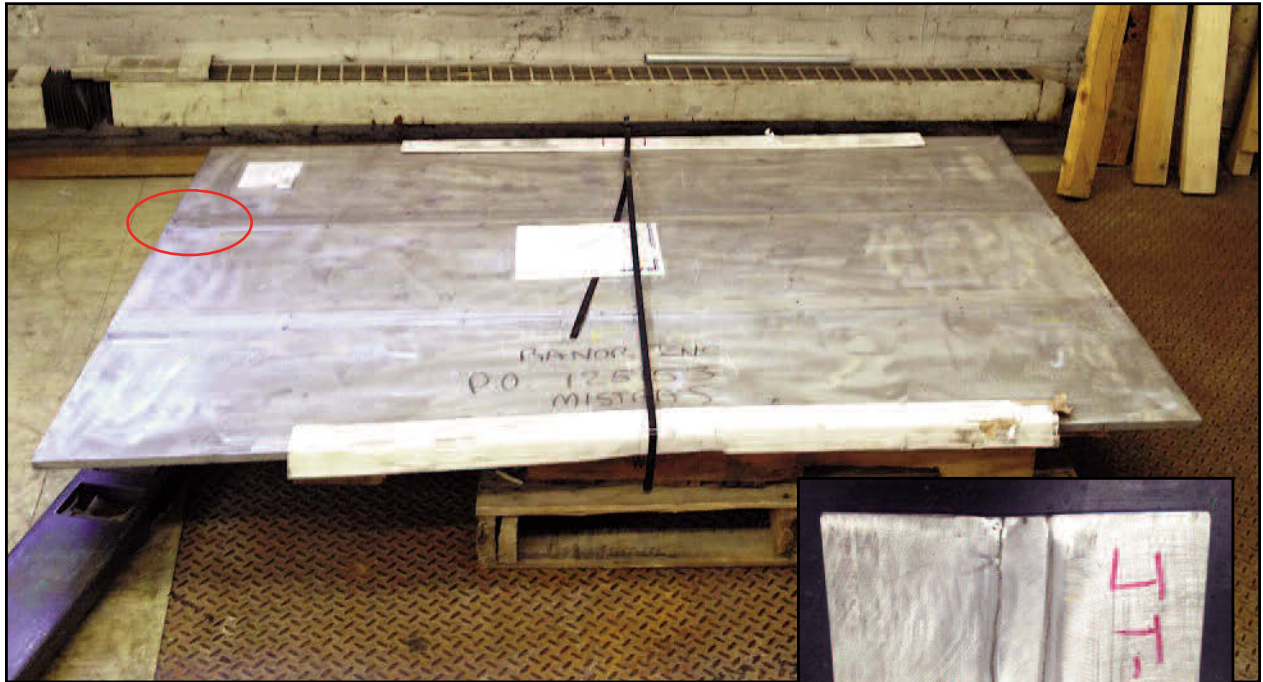
Fig. 4. The as-received flat-plate welds, November 2013. A section of the flat-plate weld (inset) was cut for microstructural analysis from the end of each weld.
