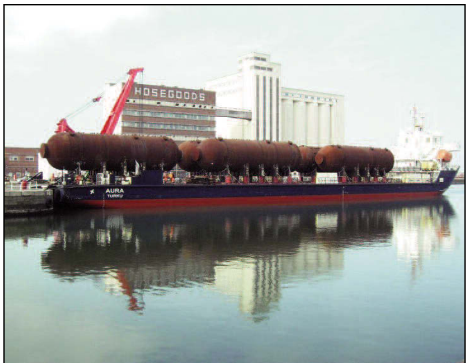
Fig. 4. Five of the Berkeley boilers, transferred to a seagoing ship and ready for transport to Studsvik's facility in Sweden. (Photo: ALE)
