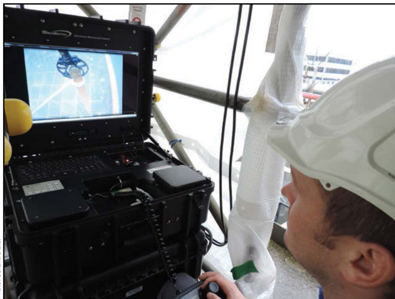
A Sellafield worker manipulates an ROV to recover cobalt isotope cartridges from a storage pond.
