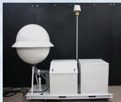
ULTRA High Volume CTBTO Air Sampler
