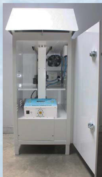
MEGA High Volume Air Sampler
